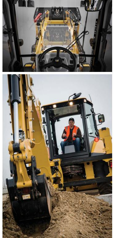
The 428F2 is fitted with mechanical controls providing low effort operation, with the ability to choose between ISO (Excavator) or SAE (Backhoe) control patterns. Providing easy and safe operation for operators of any experience or ability.
