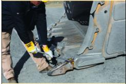
▲ A standard prying tool is used to disengage the "latch" for removal of the hammerless retainer.
