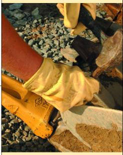
▲ The **drive-through** retainer can easily be removed from the top or bottom of the tip. Low force with a hammer and punch will disengage the retainer.
